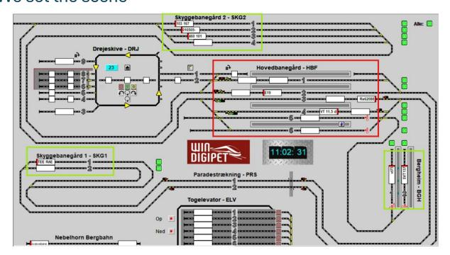
I have a main station HBF with 6 tracks, and from here, trains arrive at and depart for two staging yards, SKG1 (2 tracks) and SKG2 (4 tracks), as well as to Bergheim station BGH - 2 tracks.
