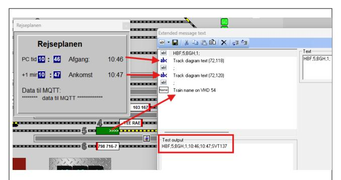
We use the Extended Text Editor to collect the required information into a text string. The individual elements are separated by ";"
