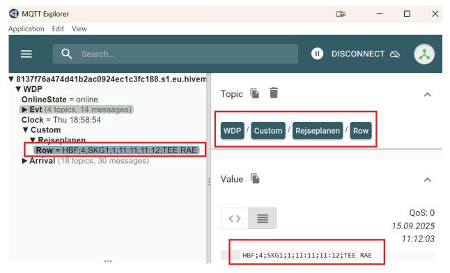
In an MQTT explorer, we can now see that data is being received from Windigipet. We always see the latest message, and the next step is to create a program that reads these messages and stores them in a table. So, we're done making changes in Windigipet and can now start building the new program, *Journey-planner*.
