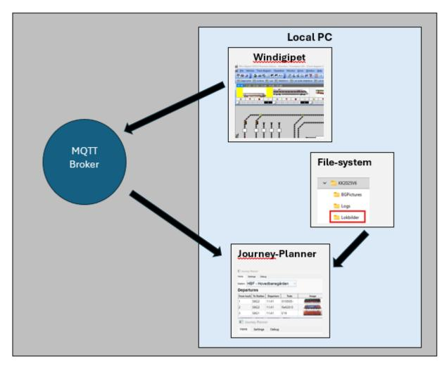
Here you can see the data flow for our new system. I'm running my MQTT broker in the cloud – but it could just as well be installed on a local PC. From Windigipet, messages are sent to the MQTT broker, and these are then picked up by our new Windows app *Journey Planner*.
