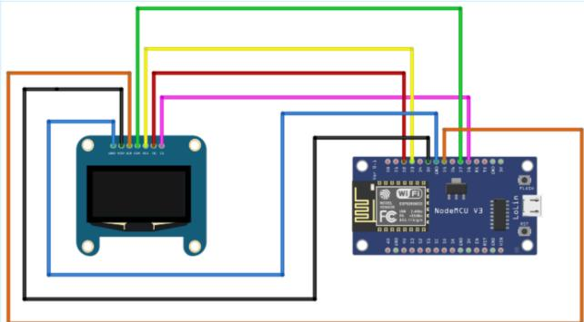
For the project, I'm using an ESP8266 together with a 0.96-inch OLED screen. They come with 7 or 4 pins. Here, I've used one with 7 pins.
