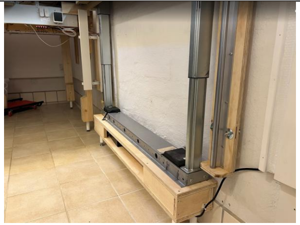
The control box for the height-adjustment functionality is now placed in the "foundation box."
