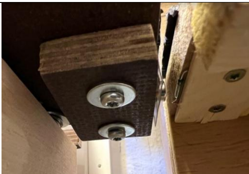
Reed switch for each track and a magnet. Connected to the S88 so the position can be determined.
