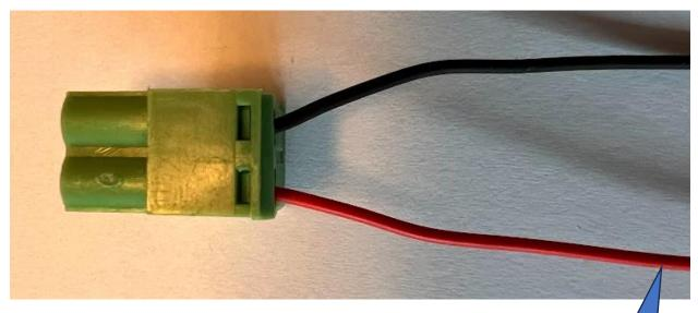
Turn the plug to the control unit correctly – for a CS2/CS3 it must be turned as shown.
