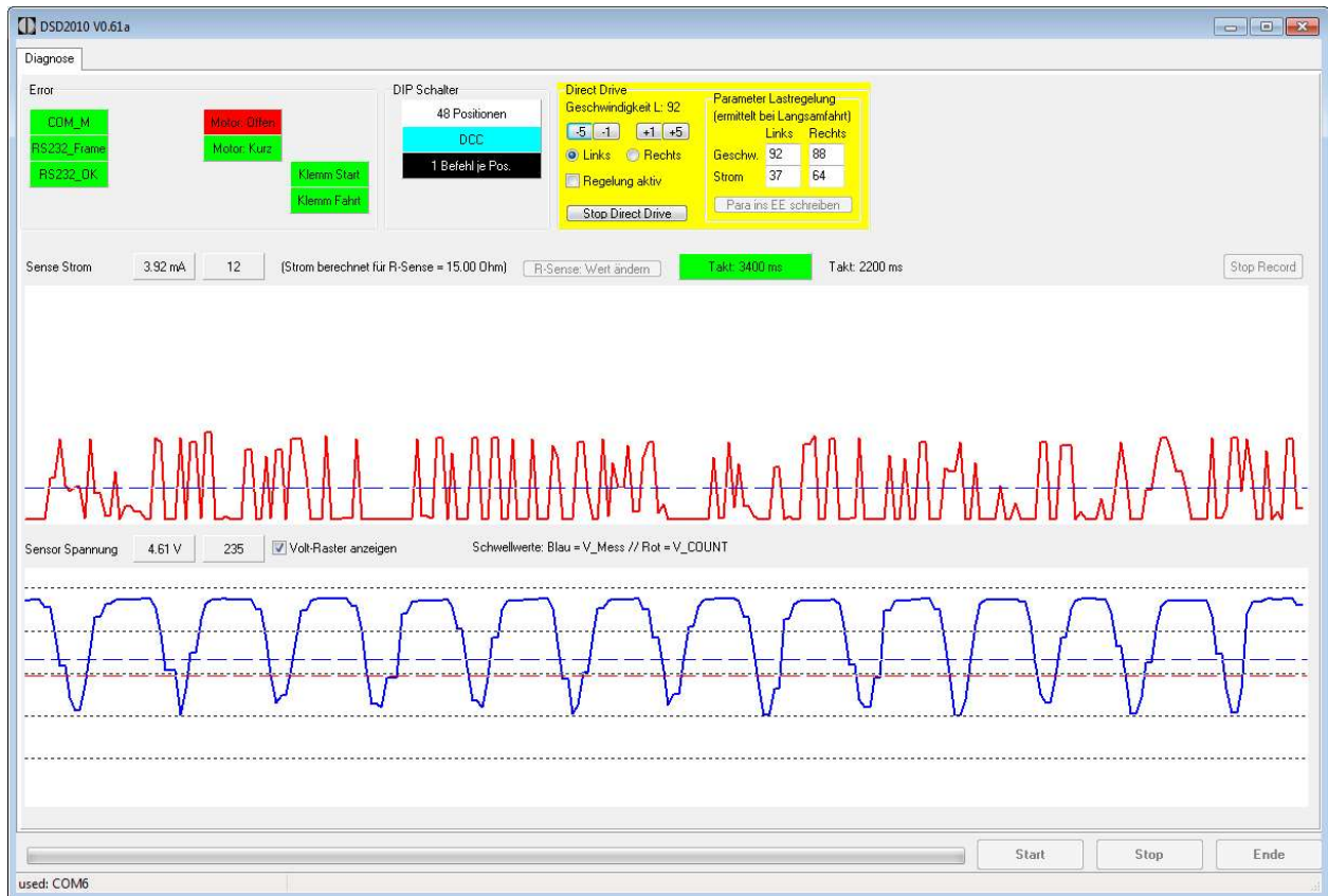
Abbildung 23: Direct Drive: Motor-Strom "zappelt"
